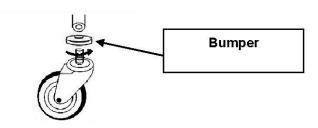
8) Put the trolley on the ground on its wheels and check that the wheels and the shelves are in the right position.
